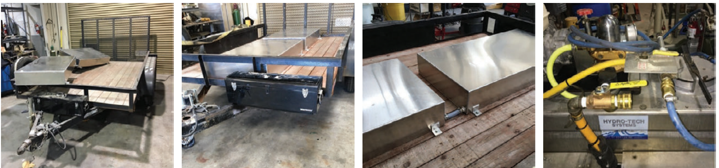
Figure 28. Nurse tank and utility box additions to the Argo trailers.
