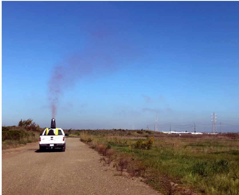
Figure 1. WALs application assessment. Truck-mounted A1 Super Duty Mist Blower applying VectoBac WDG that was dyed red for calibration purposes.
